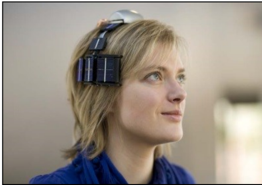
Fig. 3 Two-channel wireless EEG system with hybrid energyscavenger.
