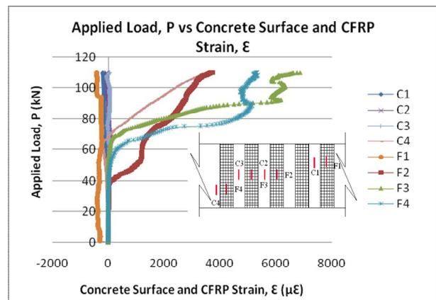
Fig. 12: Graph of Applied Load vs Concrete Surface and CFRP Strain for C2.5-UA-V2
