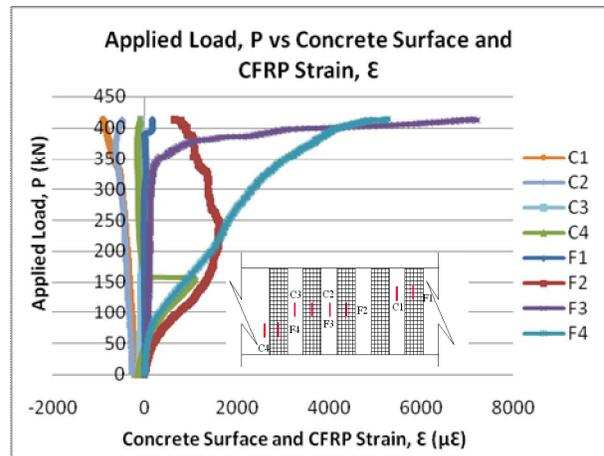
Fig. 13: Graph of Applied Load vs Concrete Surface and CFRP Strain for C2.5-U-V2
