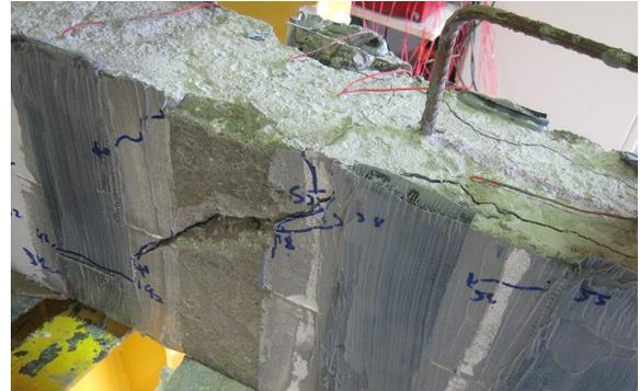
Fig. 7: Cracking and failure pattern of beam C2.5-U-V2
