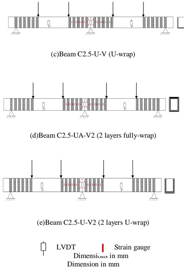
Fig. 2: Test set-up and strengthening schemes
