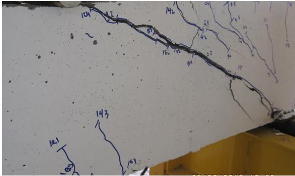
Fig. 3: Cracking and failure pattern of beam C2.5-C
