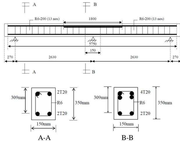
Fig. 1: Reinforcement and cross section details
