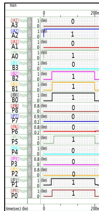
Figure 3 Output Waveform for 4x4 bit Vedic Multiplier
