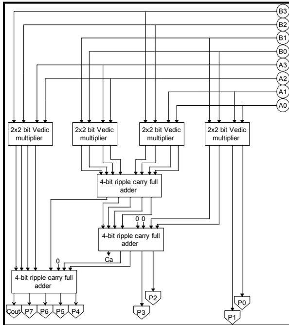
Figure 2 Block Diagram for 4x4 bit Vedic Multiplier
