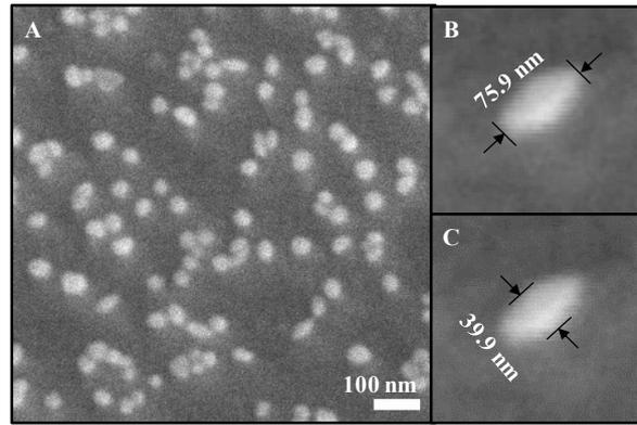
Fig. 4 FESEM image of the obtained gold nanorices grown on substrate (a) at magnification 50K, (b) single gold nanorices and its long axis size and (c) single gold nanorices and its short axis size obtained from magnification 100K.
