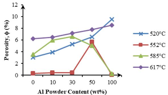
Fig. 5 The apparent porosity (%) against sintering temperatures with increasing Al powder content.
