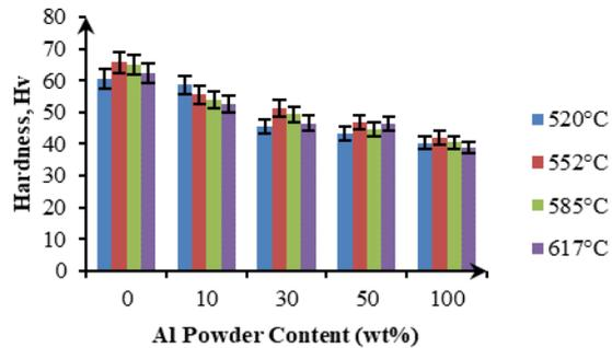
Fig. 6 The graph of hardness ( $H_V$ ) against different sintering temperatures with increasing Al powder content.
