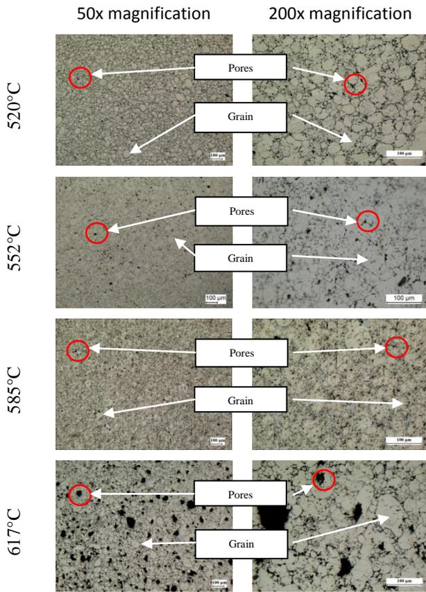
Fig. 3 The microstructure analysis of aluminium powder at four different sintering temperature
