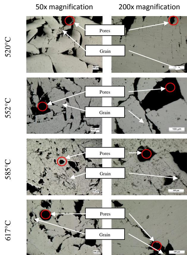
Fig. 2 The microstructure analysis of recycled aluminium (AA6061) at four different sintering temperature.
