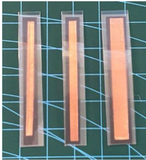
Fig. 4 Sample of 1.0mm, 3mm, and 5mm copper film on flexible sensor
