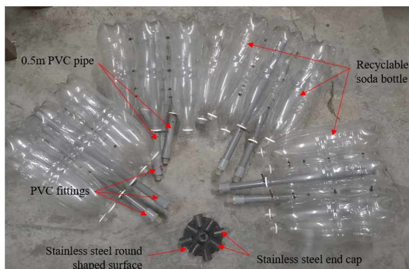
Fig. 2 Design of bottle blade for portable overshoot waterwheel
