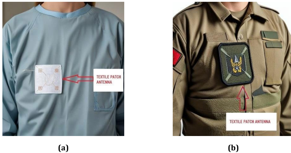
Fig. 1 (a) Textile antenna incorporated in (a) patient cloths for medical monitoring; (b) military uniforms for tracking and communication
