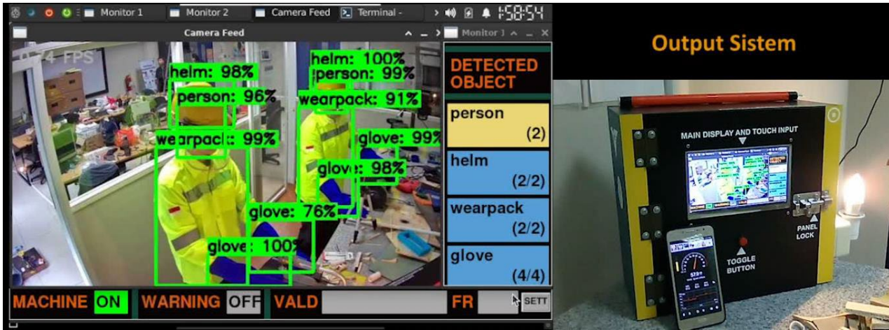
Fig. 10 Detection of multiple workers wearing PPE
