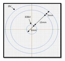
Fig. 2 Size and dimension of XLPE insulator.
