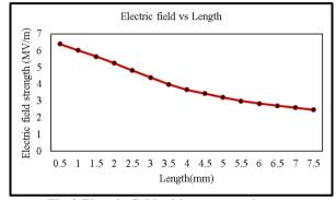
Fig.8 Electric field without contaminant.
