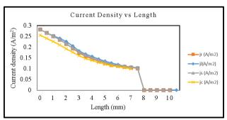
Fig.15 Comparison of current density of all conditions.
