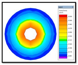
Fig. 3 Colour map and legend of current density without any contaminant.
