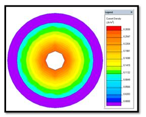
Fig. 5 Colour map and legend of current density with presence of rain water.
