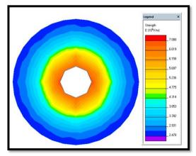
Fig. 4 Colour map and legend of electric field without any contaminant.
