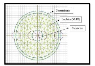
Fig. 1 Cross-sectional area of XLPE cable.
