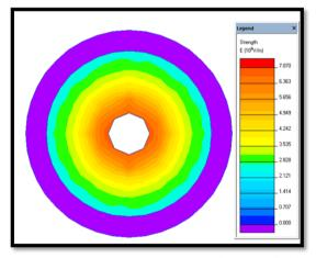
Fig. 6 Colour map and legend of electric field strength with presence of rain water.
