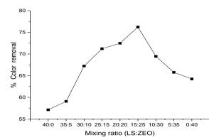
Fig.2 Percentage of color removal against different ratios of limestone and zeolite
