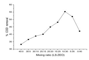
Fig.1 Percentage of COD removal against different ratios of limestone and zeolite
