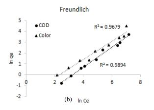
Fig.3 Plots of (a) Langmuir and (b) Freundlich isotherms for COD and color adsorption onto LS-ZEO
