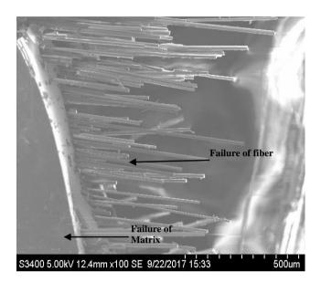
Fig.8.a - Micrograph of EGM0 sample after impact test
