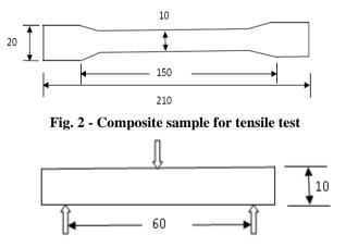
Fig. 3 - Composite sample for Flexural test
