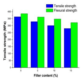
Fig. 6 - Tensile strength and Flexural strength of composite samples
