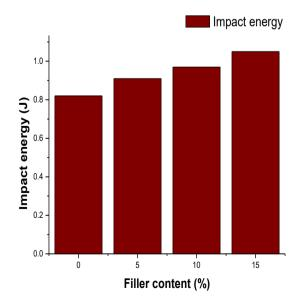
Fig. 7 - Impact energy of composite samples
