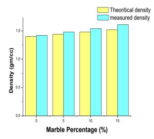
Fig. 5 - Theoretical measured densities of composite samples
