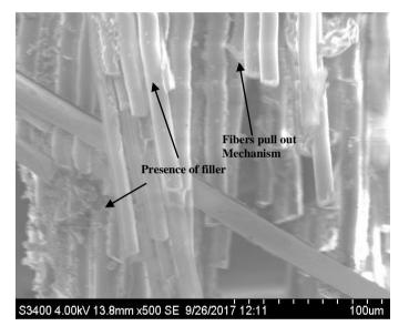
Fig.8.d - Micrograph of EGM0 sample after tensile test
