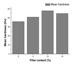
Fig. 5 - Mean hardness of composite samples
