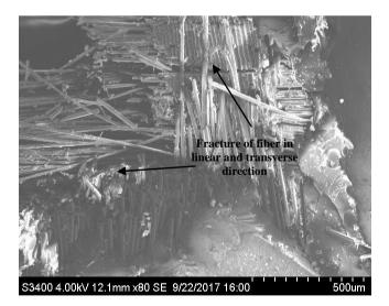
Fig.8.b - Micrograph of EGM1 sample after impact test
