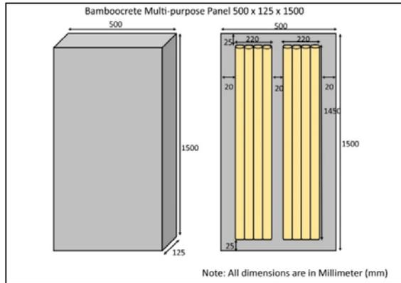
Fig. 1 Bamboocrete Multi-purpose Panel
