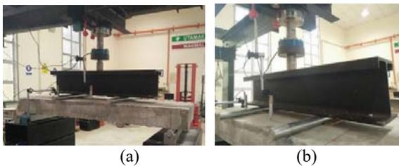
Fig. 6 Flexural Load Test. (a) General set up (b) Load cell and LVDT to capture data
