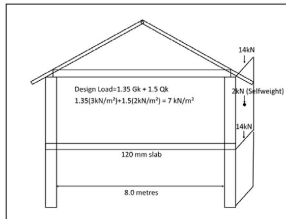
Fig. 4 Load distribution on wall panel
