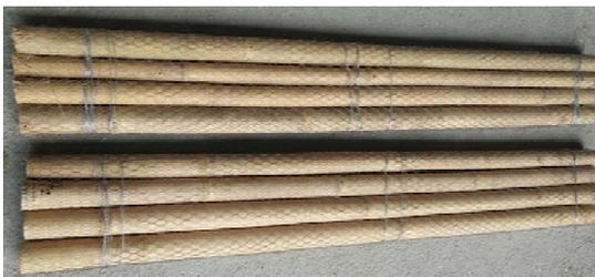
Fig. 2 Bamboo wrapped with wire mesh.
