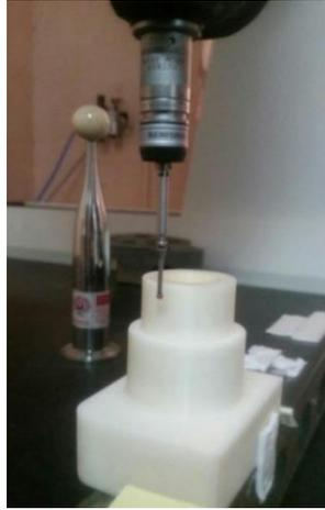
**Fig. 2 - Accurate Spectra CMM during measuring dimensions**
