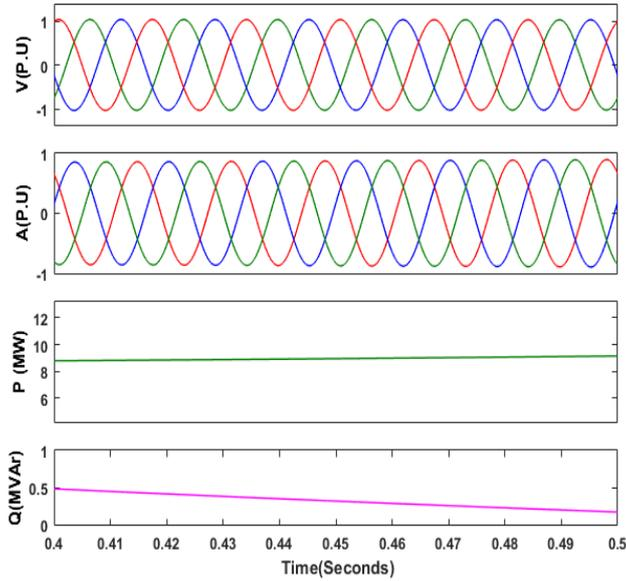
Fig.4 - Voltages, currents, active power and reactive power of grid connected operation
