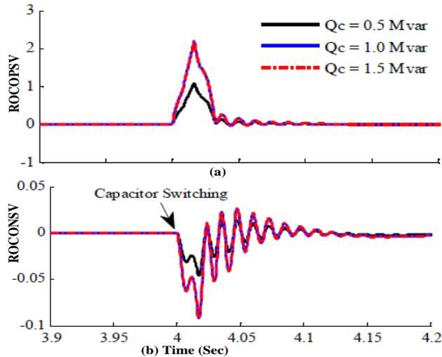
Fig. 9 - Simulation results of (a) ROCOPSV and (b) ROCOPSC during various ranges of non islanding capacitor switching.
