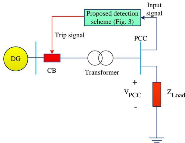
Fig. 1- Principle of islanding detection scheme
