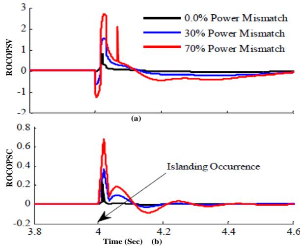
Fig. 7 - Simulation results of (a) ROCOPSV and (b) ROCOPSC with various power imbalances
