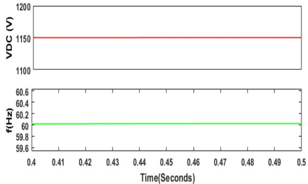
Fig.5 DC link voltage and frequency of grid connected operation
