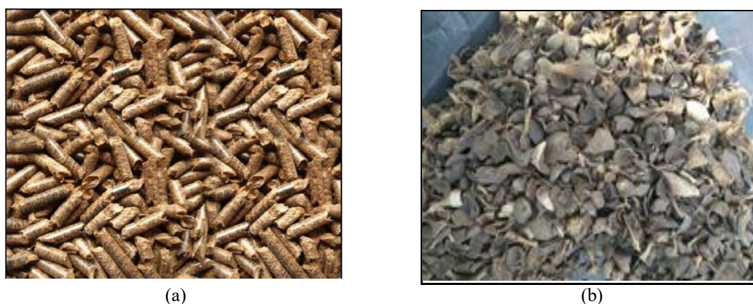
Fig. 1 - (a) empty fruit bunch pellet (EFBP); (b) oil palm shell (OPS)
