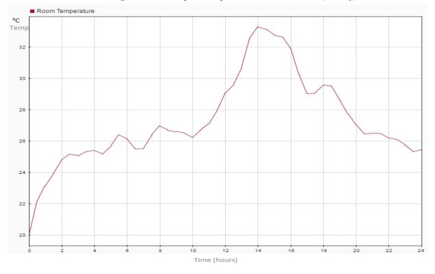
Fig. 7 – Room temperature profile with controller (hot day)
