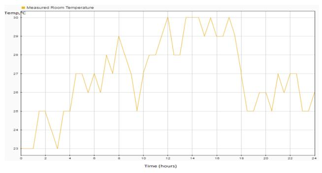
Fig. 9 – Room temperature profile without controller (cloudy day)
