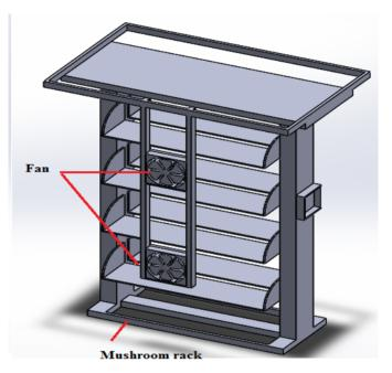
Fig. 3 – Air cooling system
