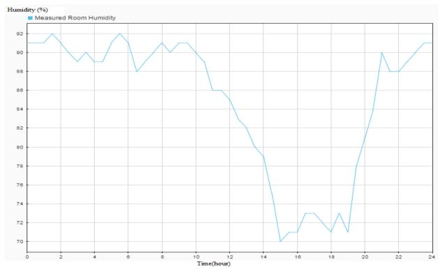
Fig. 13 –Room humidity profile without controller (cloudy day)
