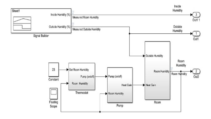
Fig. 5 – Humidity control subsystem
