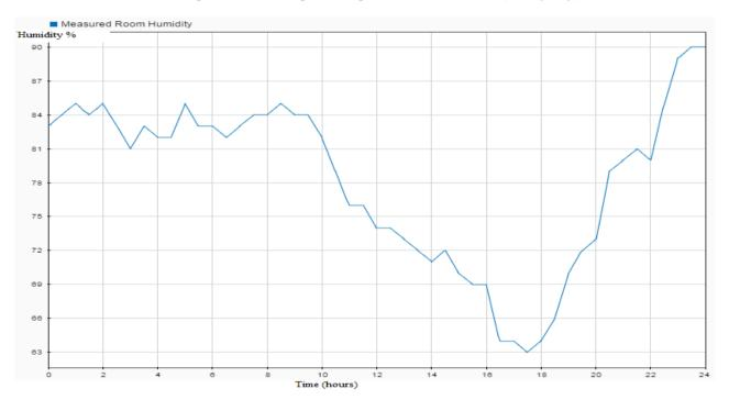
Fig. 11 – Room humidity profile without controller (hot day)
