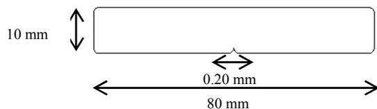
Fig 5 Sample for impact testing [8].
