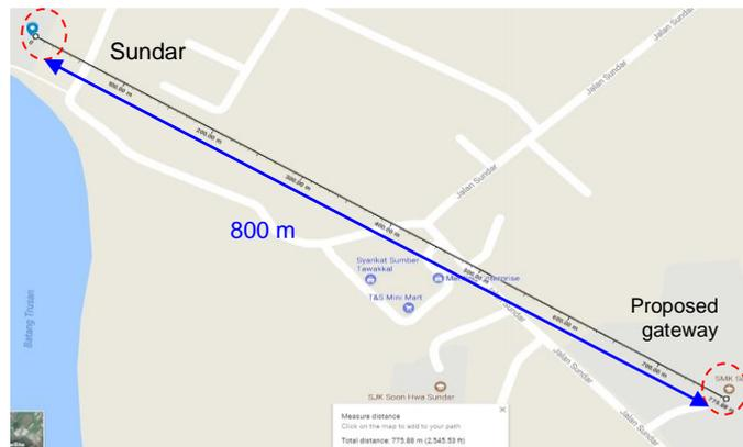
**Fig. 11– Distance of proposed gateway location to existing VSAT station (Sundar).**
