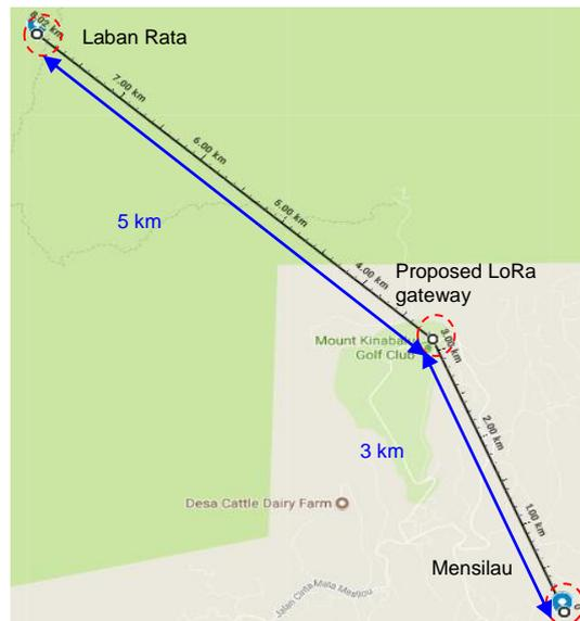
**Fig. 10–Distance of existing VSAT locations (Mensilau and Laban Rata) to proposed LoRa gateway location.**
