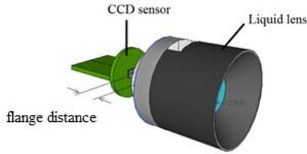
Fig. 1 Webcam CCD sensor and liquid lens assembly
