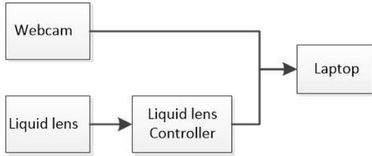
Fig. 2 Parts connection
