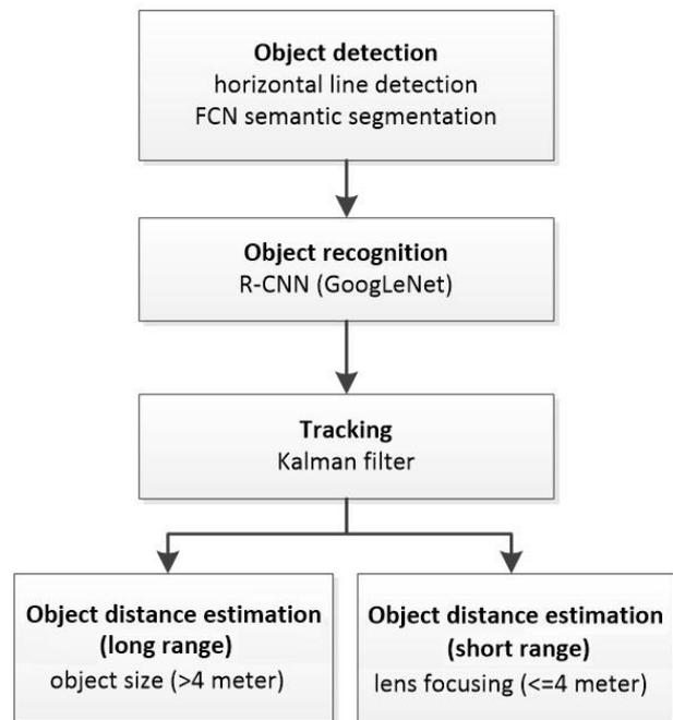
Fig. 4 Framework for oncoming vehicle detection with variable-focus liquid lens.
