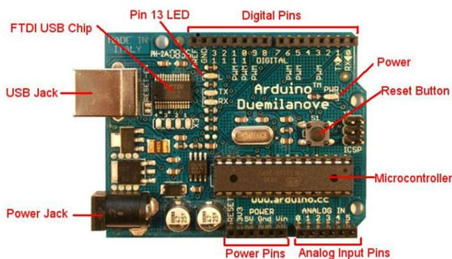
Fig. 4 Arduino circuitry board [13]
