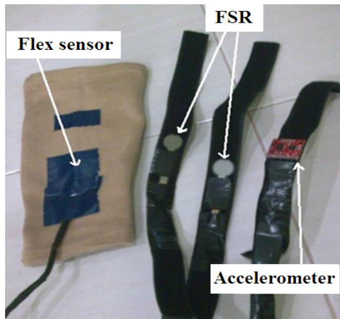
Fig. 17 Picture of sensory unit with Velcro strap.
