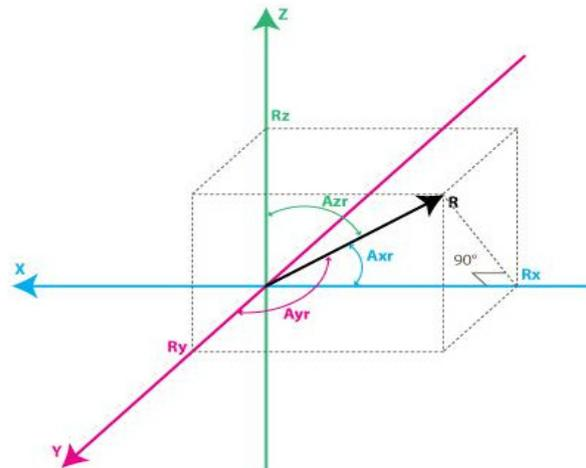
Fig. 3 A model of accelerometer axes and its correspond force vectors (Rx,Ry,Rz) and angles (Axr, Axy and Axz)[16].
