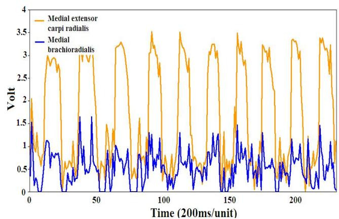
Fig. 10 Force sensitive resistor's voltage results based on object lifting activity.
