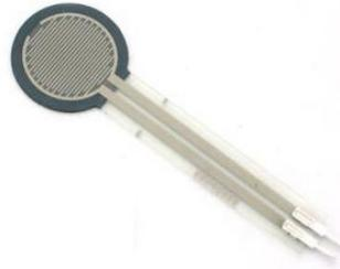
Fig. 2 Force sensitive resistor (FSR) [17]
