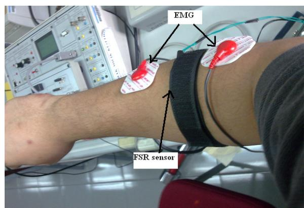
Fig. 7 Location of EMG and FSR targeted medial extensor carpi radialis on the lower arm.
