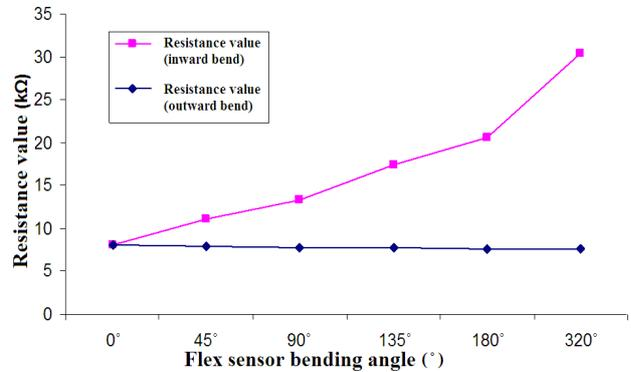
Fig. 5 Resistance value against flex sensor bending angle.
