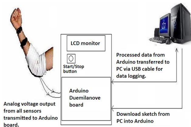
Fig. 14 Overall hardware setup diagram
