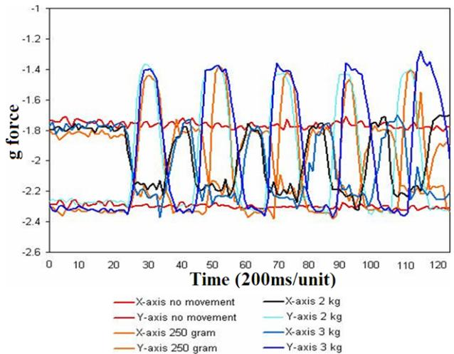
Fig. 12 Voltage output from accelerometer based on different weight during object lifting activity.
