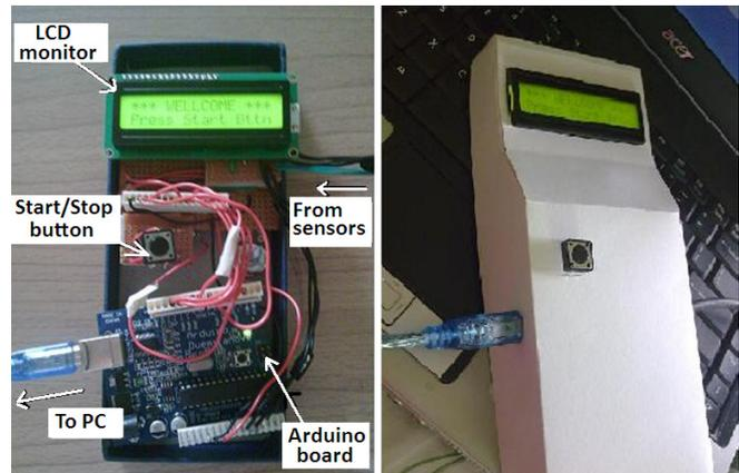
Fig. 16 Hardware setup of the main unit for the monitoring device.(a) actual main unit circuitry (b) main unit with custom built box.
