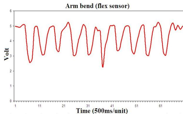
Fig. 6 Flex sensor voltage value due to arm bending movement.
