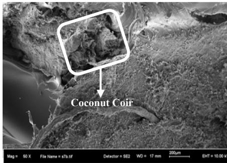
Fig.5b. Magnification at Mixture of 90 wt. % LDPE, 10 wt. % coconut coir.
