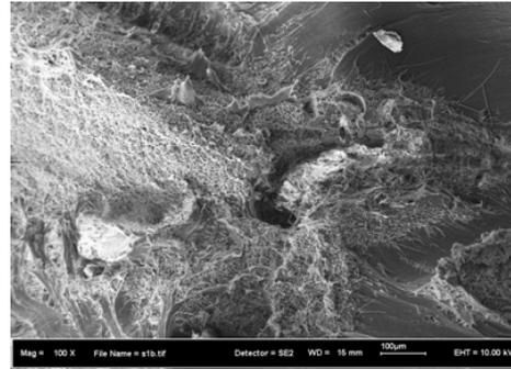
Fig.3a. Magnification at Mixture of 90 wt. % LDPE & 10 wt. % wax.
