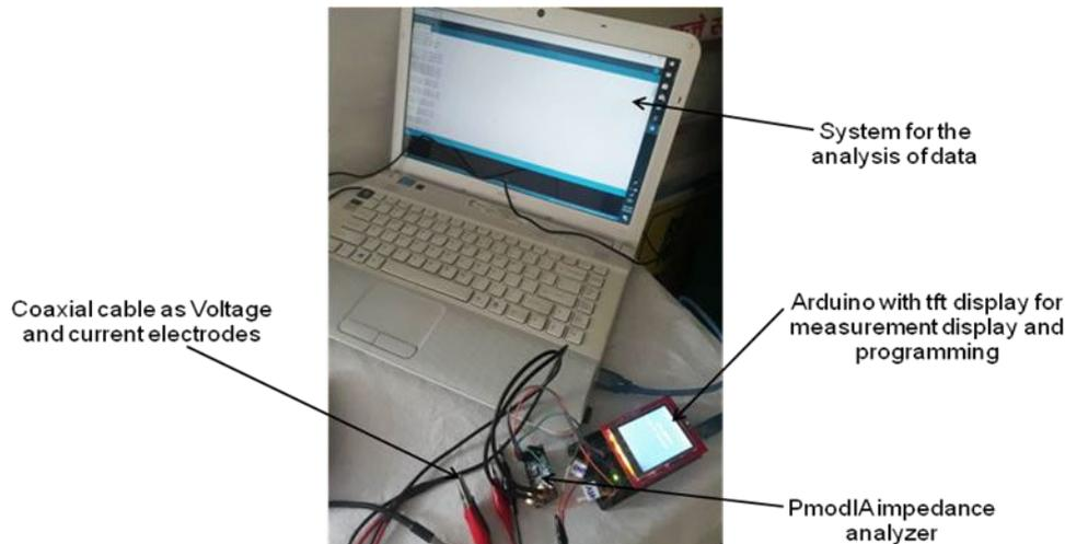
**Fig. 5 - Experimental set up for the impedance measurement system**
