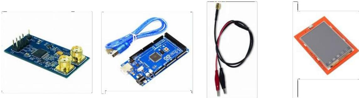
**Fig. 6 - (a) PmodIA impedance analyzer; (b) Arduino microcontroller; (c) SMA to alligator coaxial cable; (d) TFT LCD screen**
