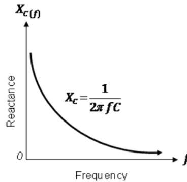
**Fig. 3 – Capacitive Reactance against Frequency**
