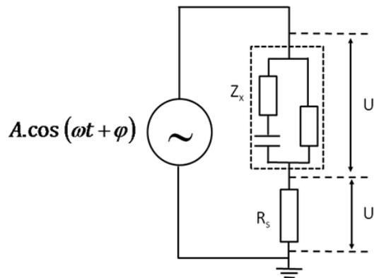
**Fig. 2 - Model of bioelectrical impedance measurement**
