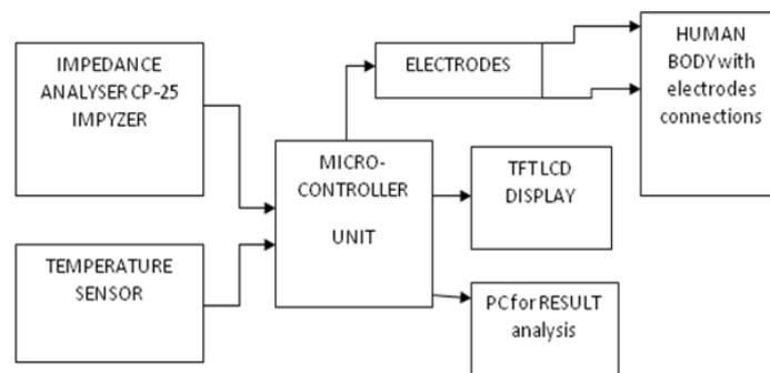
**Fig. 4 - Block diagram of proposed system**
