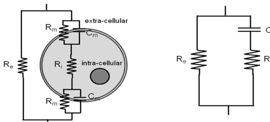
Fig.1 - (a) Model of bioelectrical impedance measurement with intra cellular water and extra cellular water; (b) Basic model of body's equivalent circuit [4]
