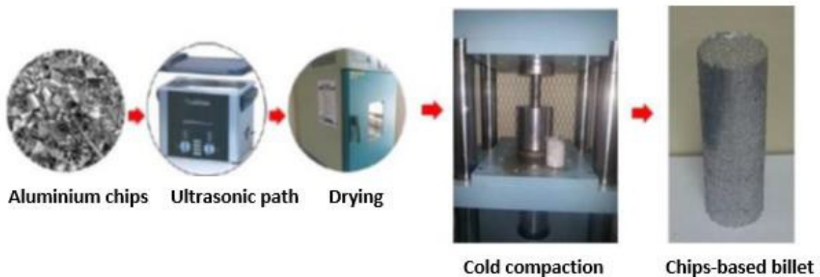
Fig. 1 - Preprocessing of chips before consolidation
