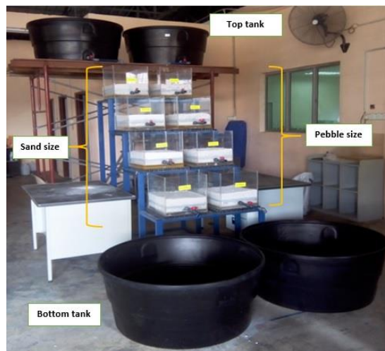
Fig. 1 - Marble filter experimental setup
