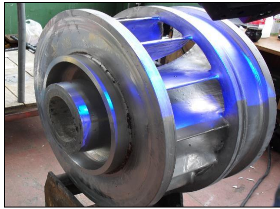
Fig. 13 - Scan face pressure Francis runner
