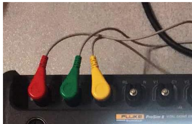
Fig. 15– Electrode placement for ECG measurement testing
