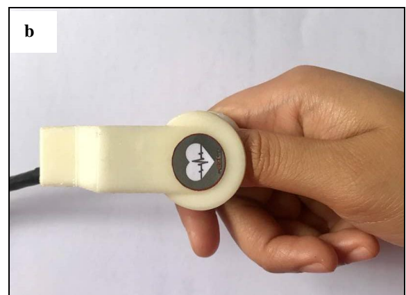
Fig. 6- (a) Body temperature measurement; (b) Blood oxygen saturation measurement
