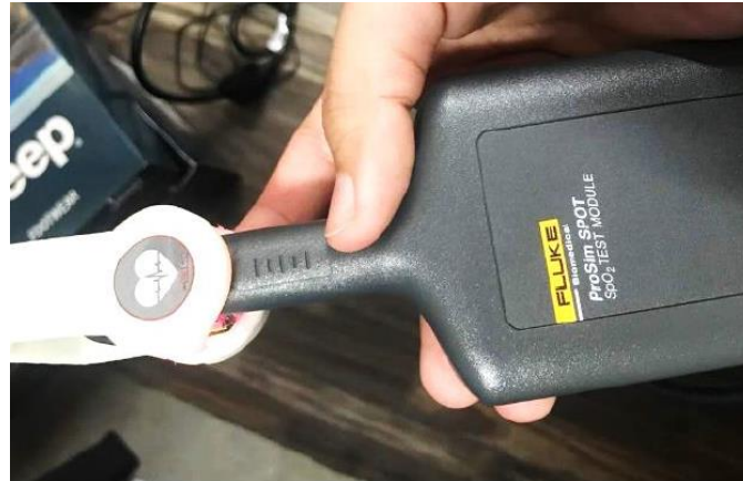
Fig. 14 - Oxygen saturation measurement testing
