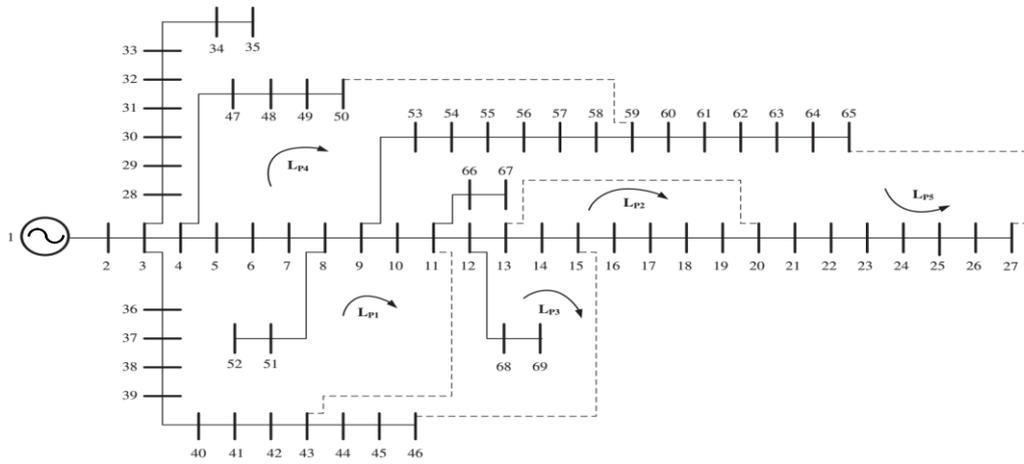
**Fig. 5- The single line diagram of 69-bus test system[20]**
