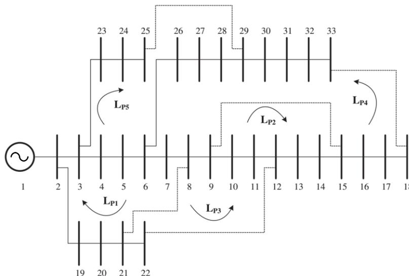
Fig. 1- The single line diagram of 33-bus test system[18]
