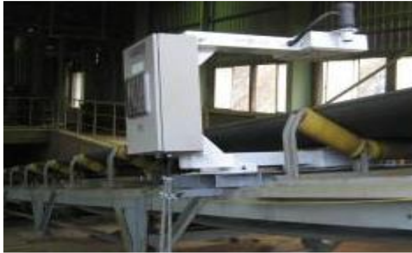
Fig.2 - Application of Microwave moisture analyzer of ferronickel
