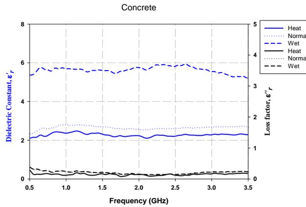
**Fig. 11 - Dielectric properties of concrete**
