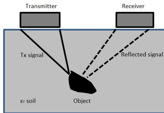
**Fig. 1 - Bi-Static GPR System**
