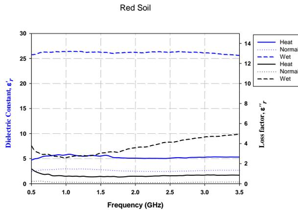
Fig. 12- Dielectric properties of red soil
