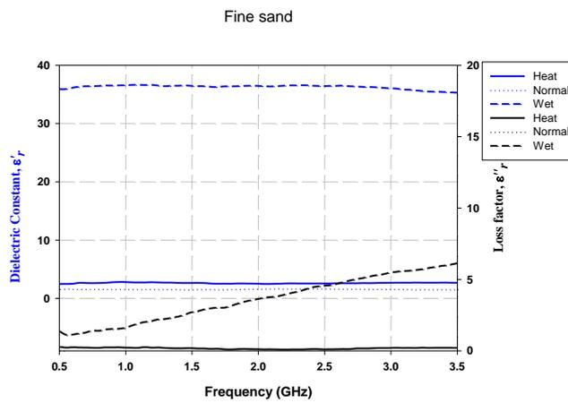
**Fig. 10 - Dielectric properties of fine sand**
