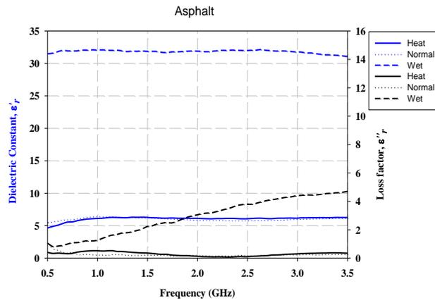
**Fig. 6 - Dielectric properties for asphalt**
