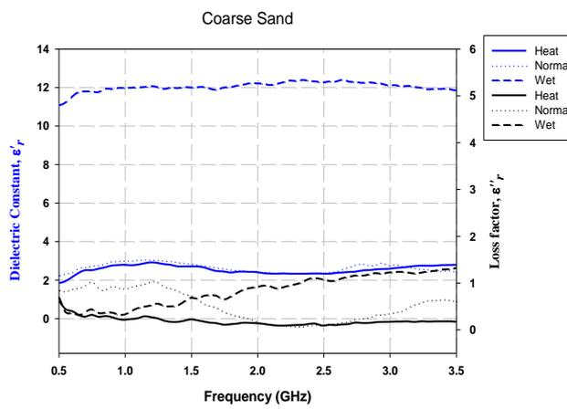
**Fig. 7 - Dielectric properties of coarse sand**
