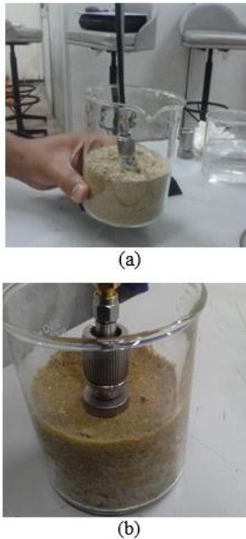
**Fig. 5 - Measured samples, (a) Dried sand (b) Wet sand**
