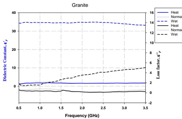
**Fig. 8 - Dielectric properties of granite**
