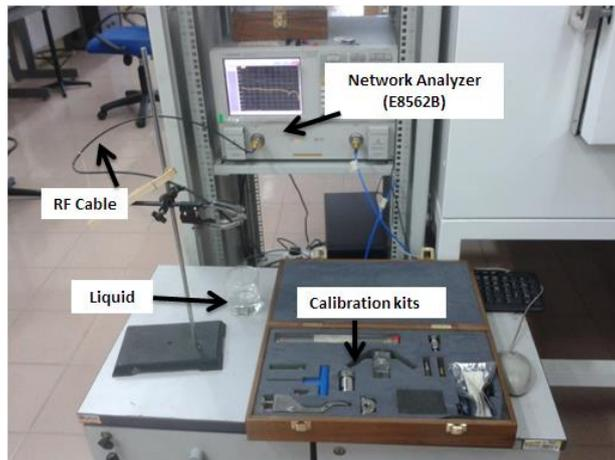
**Fig. 4 - Dielectric Coaxial Probe and Calibration Kits**
