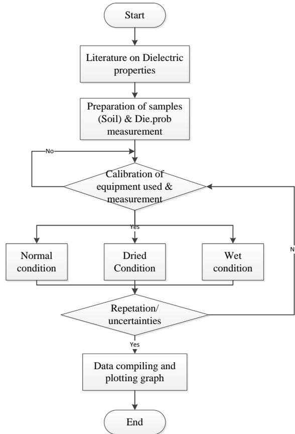
**Fig. 3 - Measurement process of dielectric characterization of soil.**
