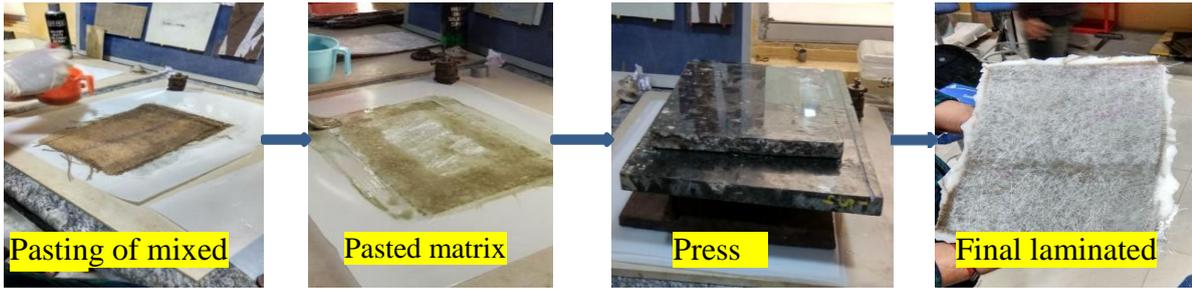
Fig. 2 - Fabrication of composite laminate
