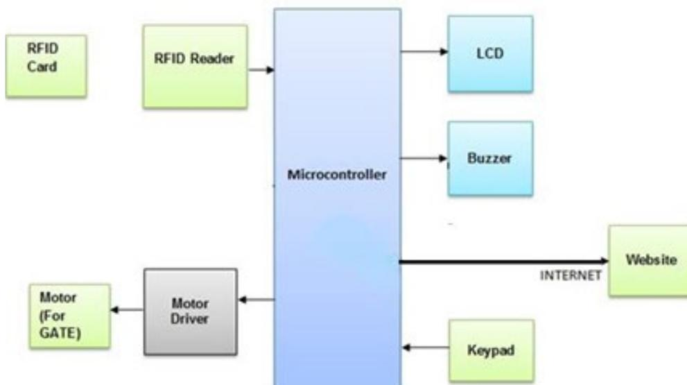
Fig. 2 - Block diagram representing the overall system
