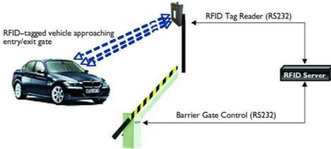
Fig. 1 - RFID barrier gate control
