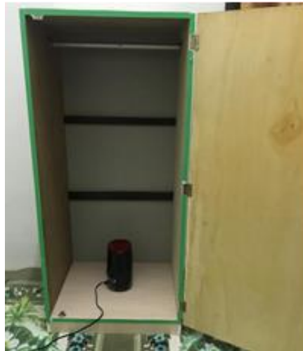
Fig. 1 - DC prototype install with dehumidifier reactor
