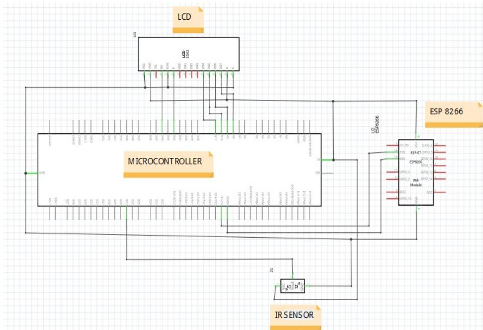
**Fig. 3 - The hardware development of the IoT-based monitoring system in the assembly line for car inner rear side body parts welding section**
