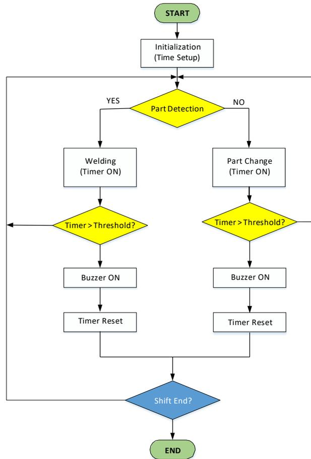
**Fig. 4 - Flowchart Production Line Worker Monitoring System**
