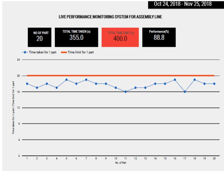
Fig. 5 - GUI of an online dashboard for assembly line monitoring system
