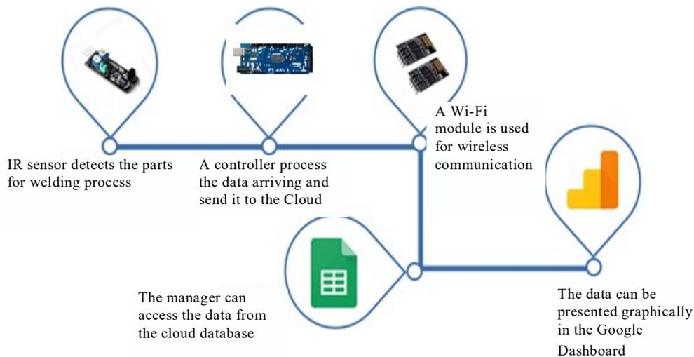
**Fig. 2 - Block diagram of the overall production monitoring system**
