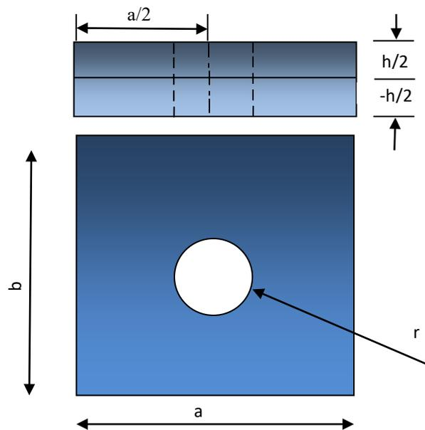
Fig. 1 - Elevation and plan of functionally graded plate with central hole
