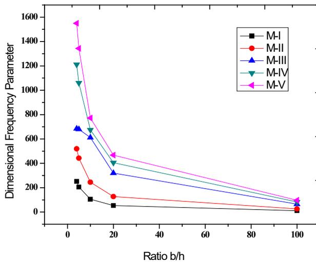
Fig 5 - Vibration responses of first 5modes of CFFF FG square plate (Ti-6Al-4V/ZrO<sub>2</sub>) with central hole  $r=0.1, q=2 T_c=500K$
