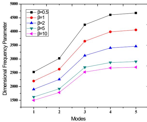
Fig 11 - Frequency parameter of first 5modes of C/SCS FG square plate (Ti-6Al-4V/ZrO<sub>2</sub>) with central hole  $r=0.1, b/h=2 T_c=500K$
