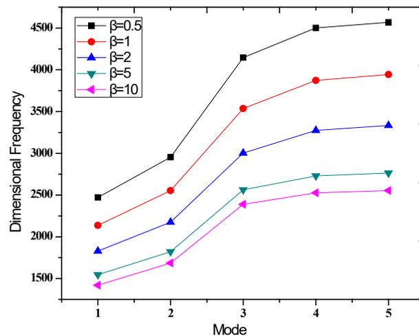
**Fig 12 - Frequency parameter of first 5 modes of CSCS FG square plate (Ti-6Al-4V/ZrO<sub>2</sub>) with central hole  $r=0.1$ ,  $b/h=2$   $T_c=700K$**
