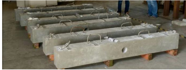
Fig. 7 - Beams after detached from formwork.
