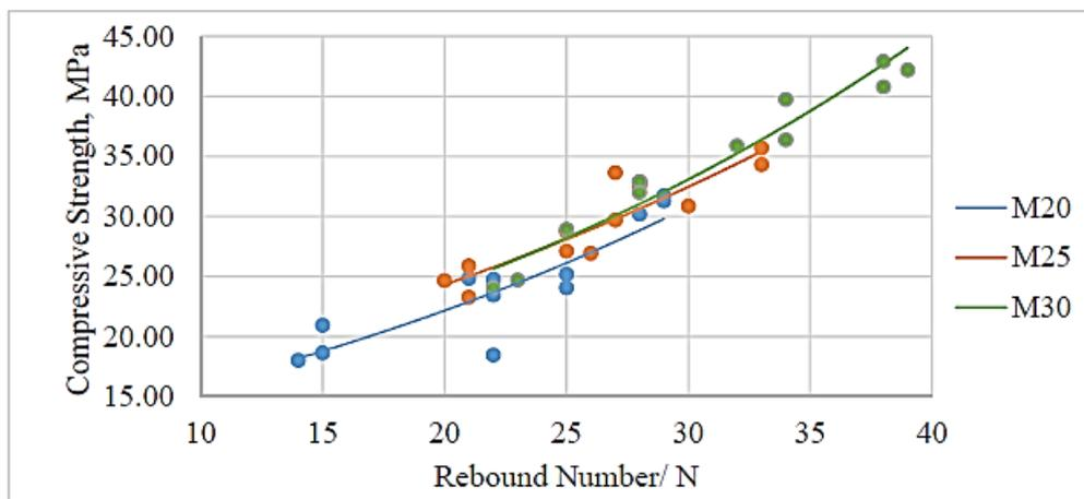
**Fig. 12 - Combined calibration curve of compressive strength of M20, M25 and M30 test against rebound number**
