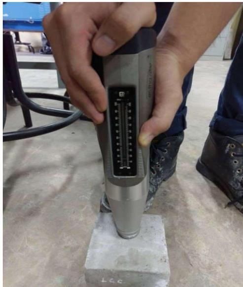
**Fig. 8 - Application on concrete surface**
