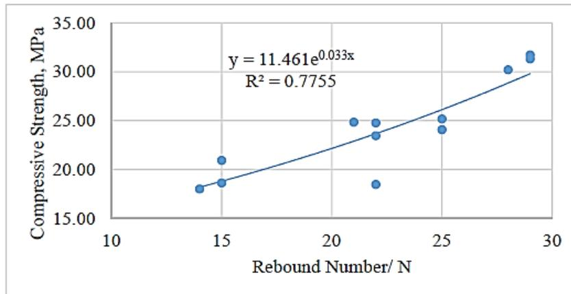
**Fig. 9 - The calibration curve of the compressive strength of M20 test vs rebound number**
