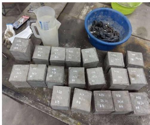
**Fig. 5 - Casting and labelling the samples**
