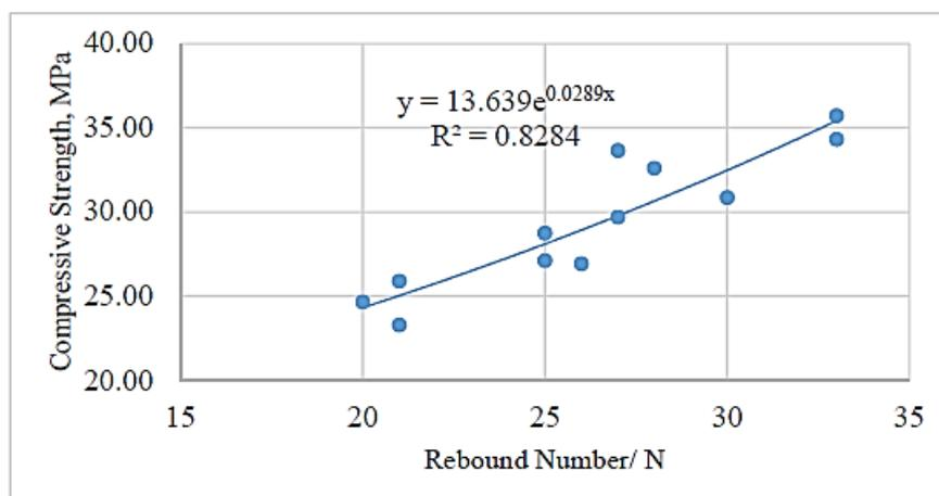
**Fig. 10 - The calibration curve of compressive strength of M25 test vs rebound number**
