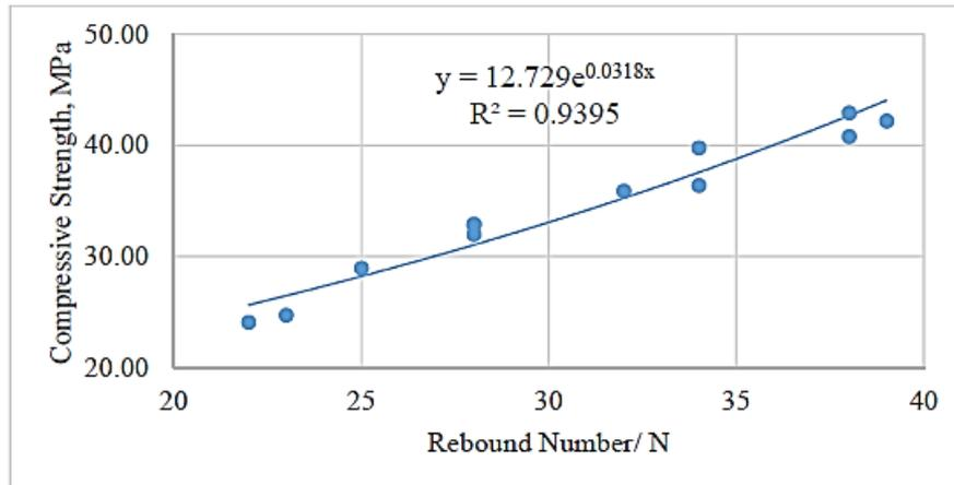
**Fig. 11 - The calibration curve of compressive strength of M30 test vs rebound number**
