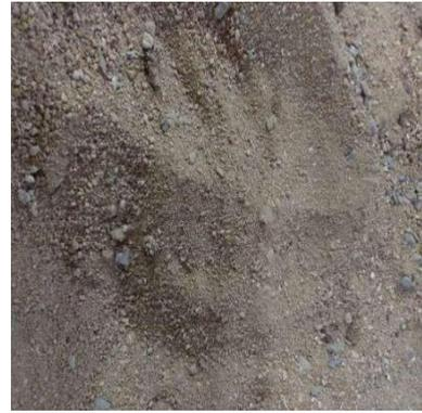
**Fig. 3 - Sand (fine aggregate)**
