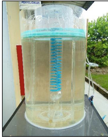
Fig. 6 - Full lab-scale GATS fabricated using acrylic cylinder tube
