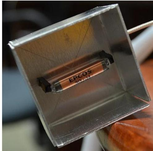
Figure 1 - Excitation coil mounted to a square-type electromagnetic screen
