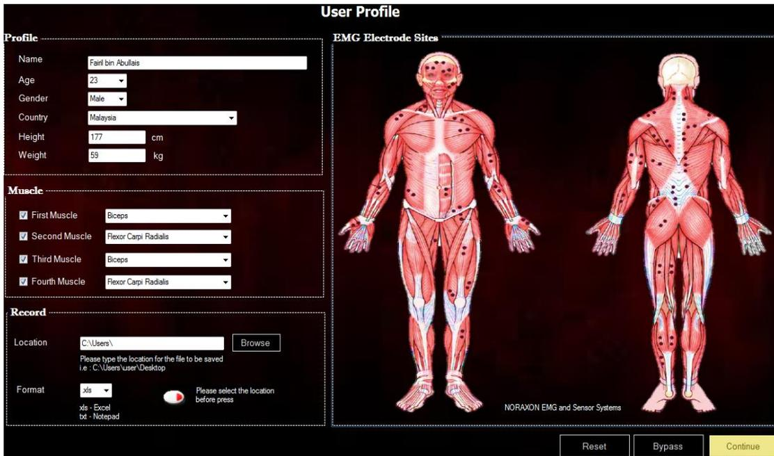
Fig. 2 - First GUI: Individual particulars, muscle measured, record and EMG electrode
