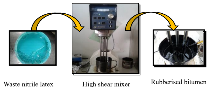
Fig 1 - Bitumen modification process using mechanical high shear mixer
