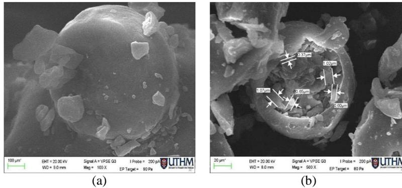
**Fig. 3 (a) - SEM of CBA (100µm), and (b) – SEM of CBA (20µm)**
