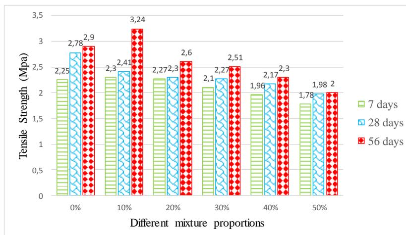
Fig. 7 - Splitting tensile strength of different replacement percentage of CBA
