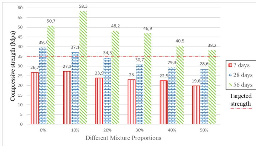
Fig. 6 - Compressive strength of different replacement percentage of CBA
