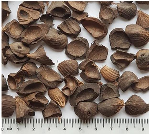
**Fig 1. - Oil palm shell lightweight aggregate**
