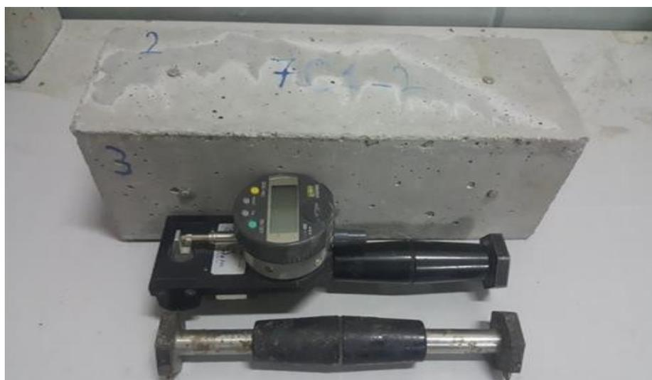
Fig. 4. The drying shrinkage measurement tool
