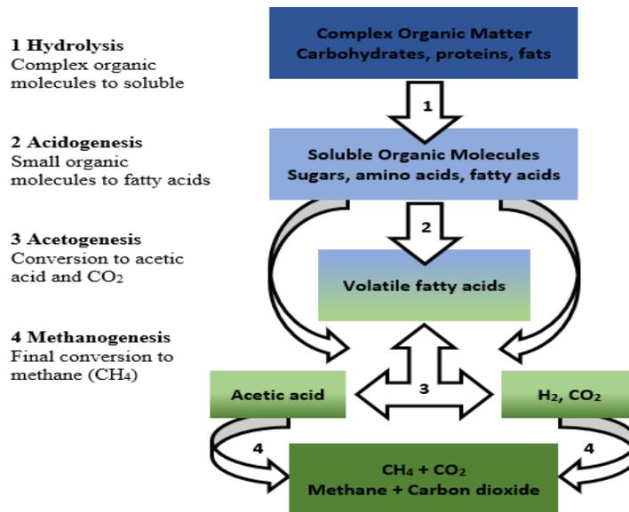
Fig. 1 - Biogas production from POME [7], [24]
