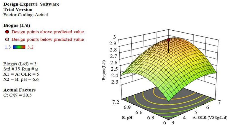
Fig. 4 - Biogas production optimization with respect to OLR and pH
