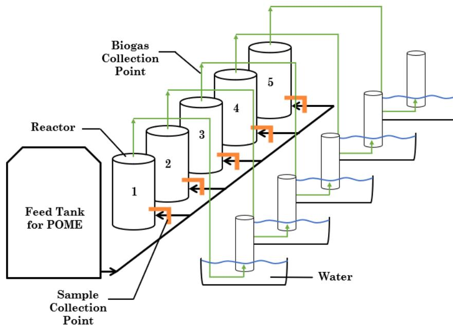
Fig. 3 - Experimental setup for biogas collection
