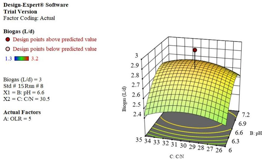
Fig. 5 - Biogas production optimization with respect to pH and C/N
