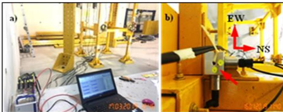
**Fig. 2 - (a) Data acquisition station; (b) Bi-axial alignment of accelerometer sensors**
