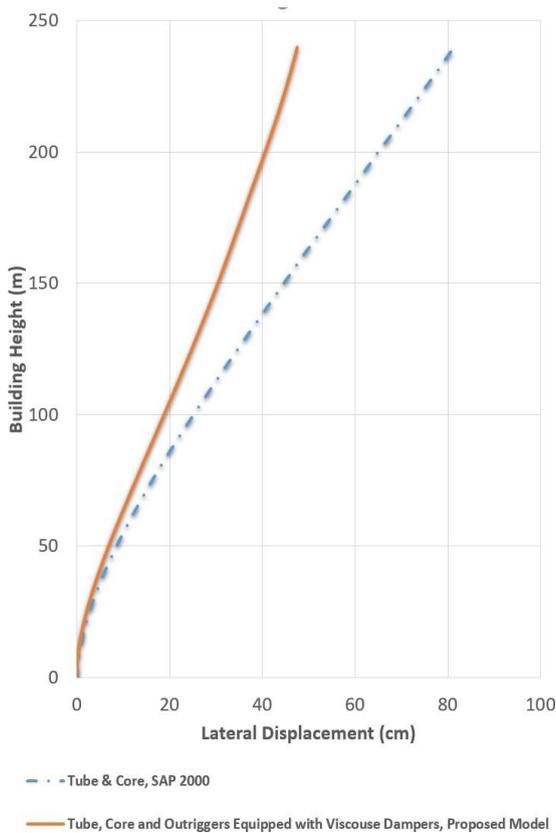
**Fig. 16 - Lateral displacement comparison of 60 story hybrid system with tubular and shear core system**
