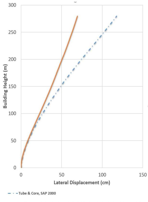
**Fig. 17 - Lateral displacement comparison of 70 story hybrid system with tubular and shear core system**
