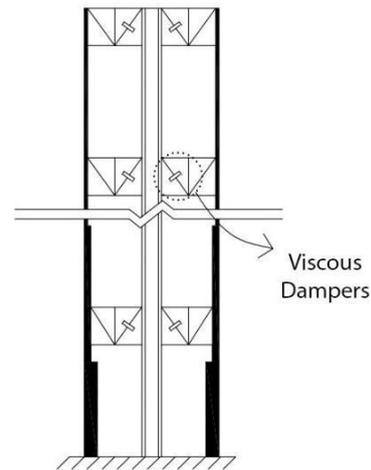
**Fig. 2 - Elevation of hybrid system with stepwise discontinuities through the height**
