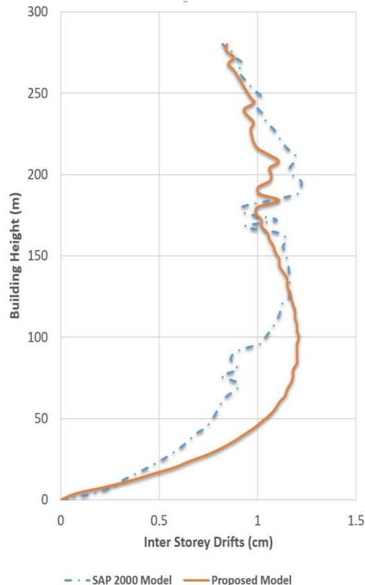
**Fig. 15 - Inter story drift profile of 70 story hybrid system**
