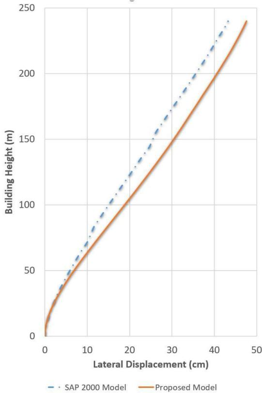
**Fig. 12 - Lateral displacement profile of 60 story hybrid system**
