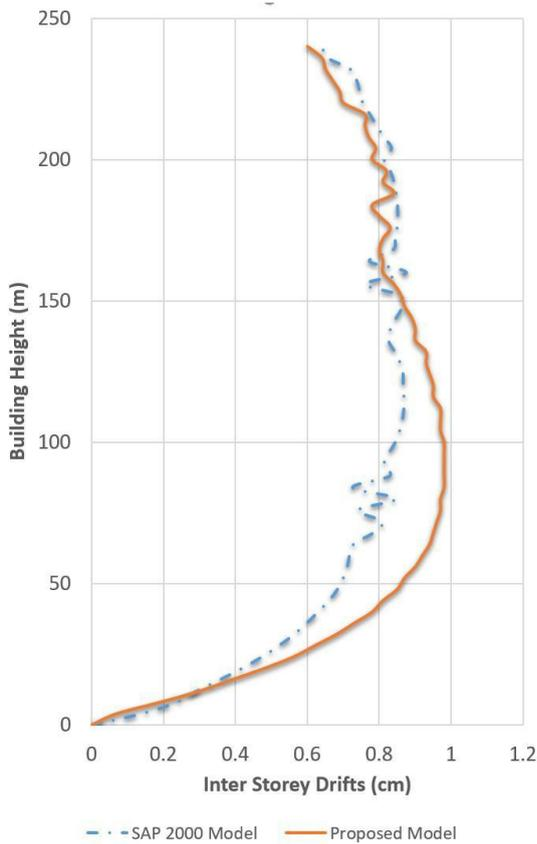
**Fig. 14 - Inter story drift profile of 60 story hybrid system**
