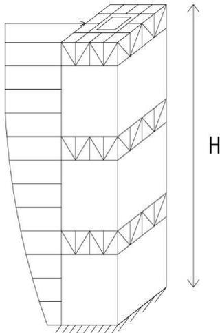
**Fig. 1 - 3D model of hybrid system**
