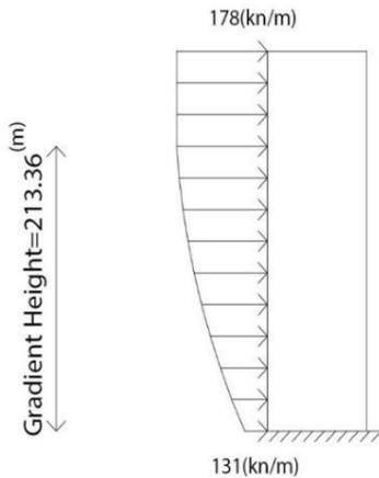
Fig. 8 - Wind load exerted on hybrid System
