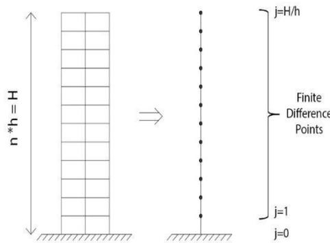
Fig. 6 - Discrete points in finite difference model
