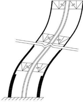
Fig. 10 - Deformed shaped of the hybrid system under lateral load
