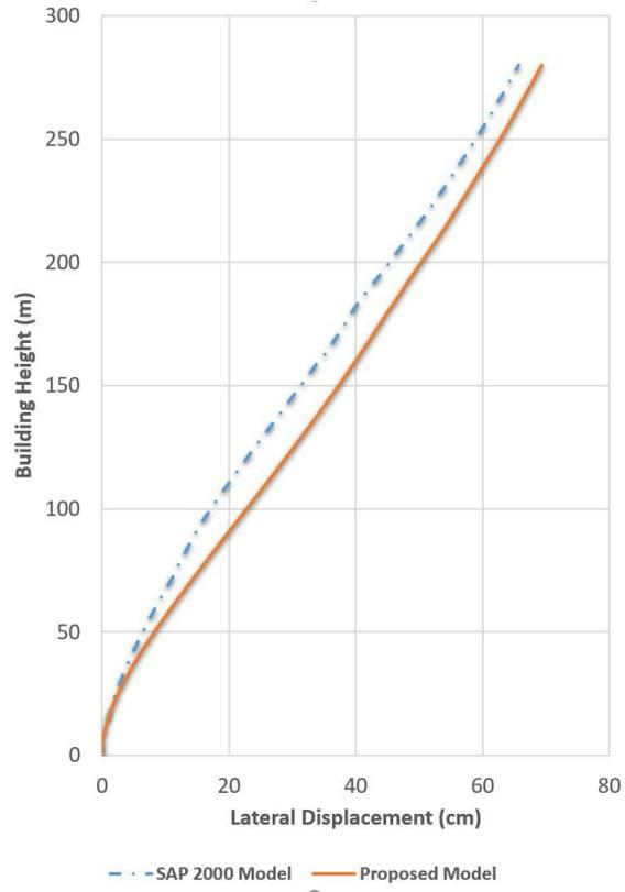
**Fig. 13 - Lateral displacement profile of 70 story hybrid system**
