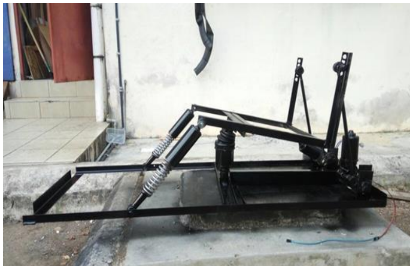
Fig. 3 - Motion simulator frame seat
