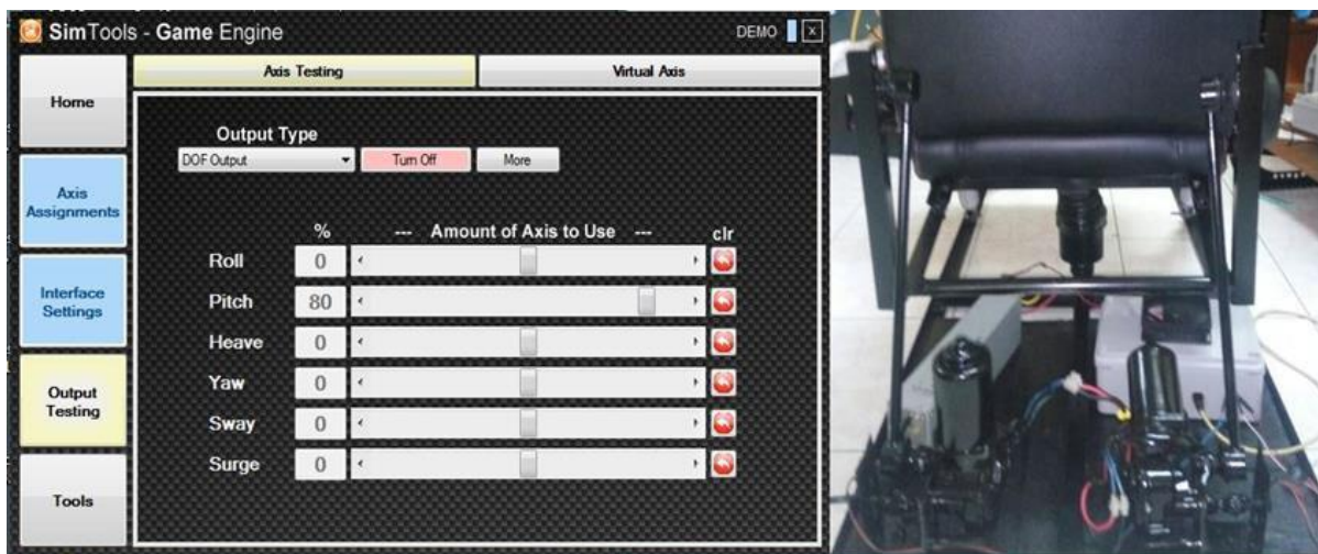
Fig. 6 (c) - The Seat Motion at +80% Roll
