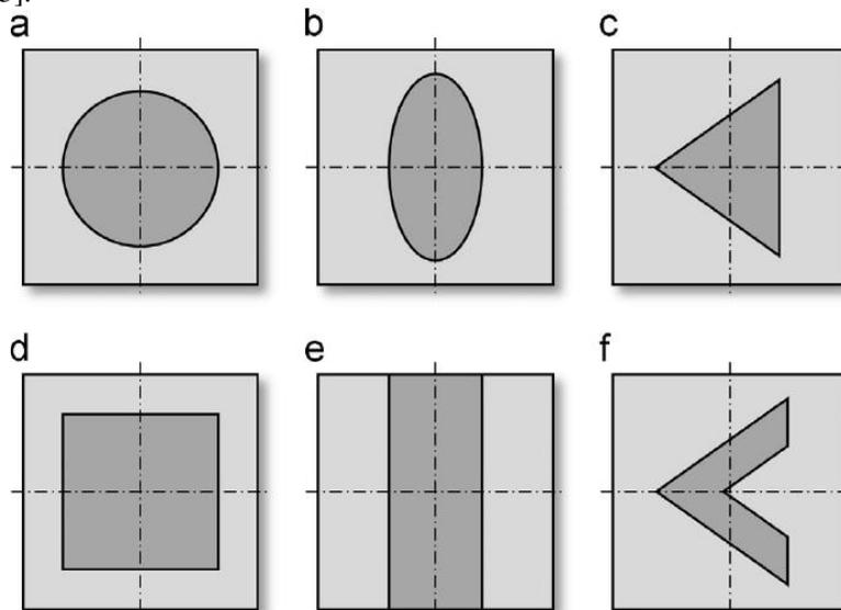
**Fig. 4 - Texture shapes. (a) circular; (b) elliptical; (c) triangular; (d) rectangular; (e) groove and (f) chevron-like [26]**
