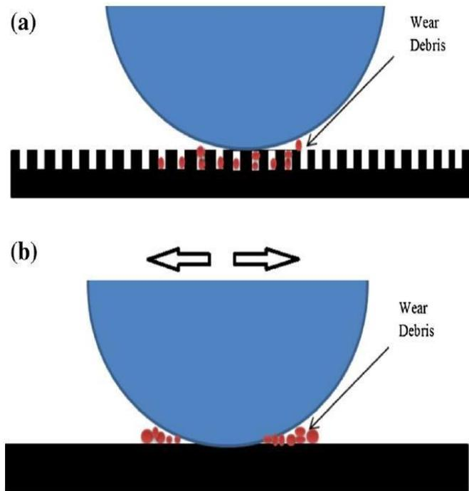
**Fig. 1 - Cross-sectional view of reciprocating ball on a plate in lubricated condition. (a) Textured surface; (b) untextured surface [8]**
