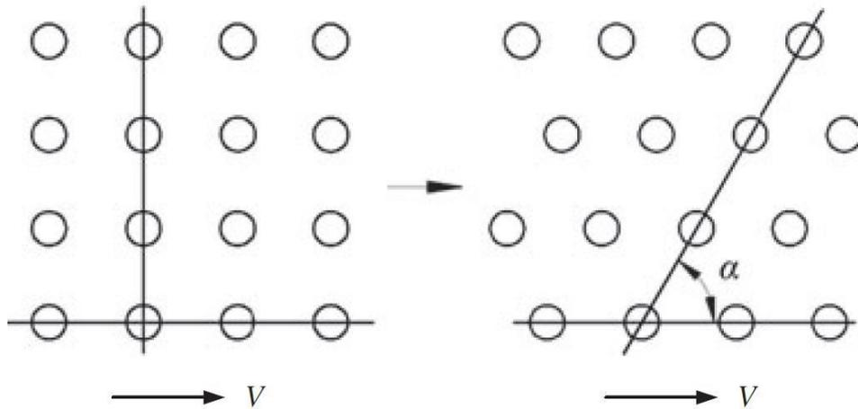
**Fig. 6 - Dimple distribution array from normal square to shifted  $\alpha$  degree array [44]**
