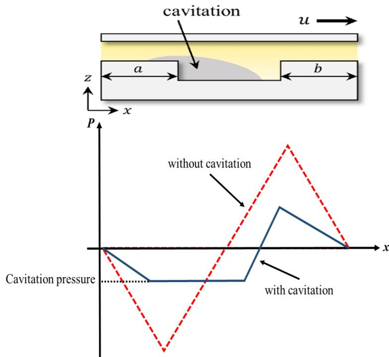
**Fig. 2 - Cavitation in a single texture cell and the pressure distribution [26]**
