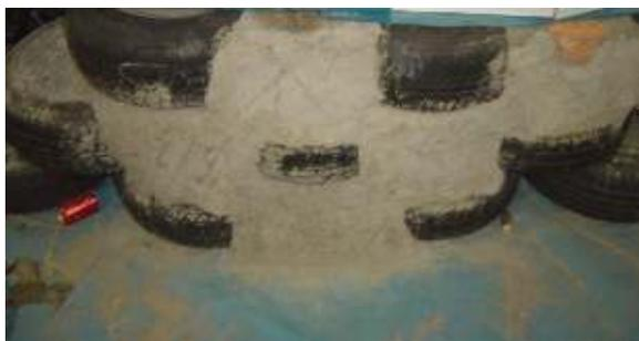
Fig. 18 Retaining Wall with Recycled Tyres
