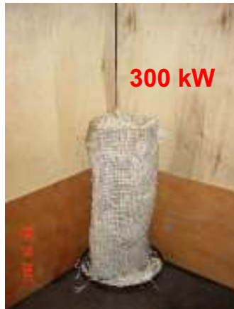
Fig. 1 Litter bin of 300 kW
